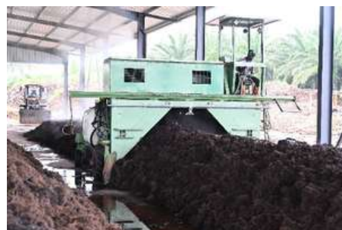
Composting machinery processing palm oil residues at the pilot site in Côte d'Ivoire. © Jacques Fuchs, FiBL
